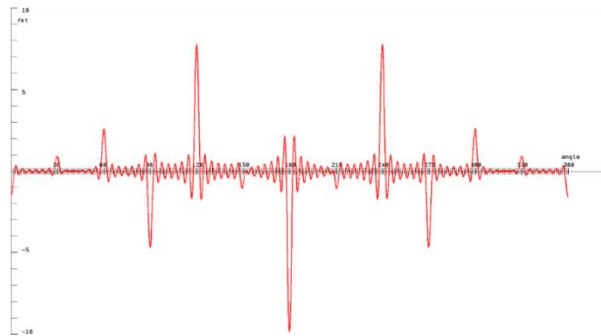
Figure 5: 7 th order correlation function H_{i,j} according to equation (10) with N = 7 . The higher orders of the correlation function are suitable for resonance problems.
